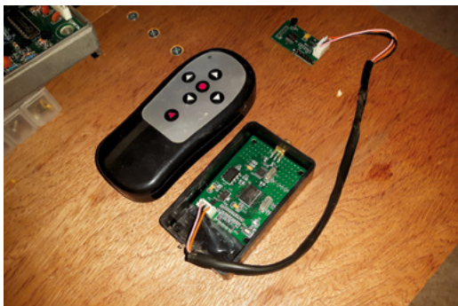
▶ The golf trolley's radio receiver was reverse-engineered so Marvin could replicate the instructions it issues using Raspberry Pi instead
