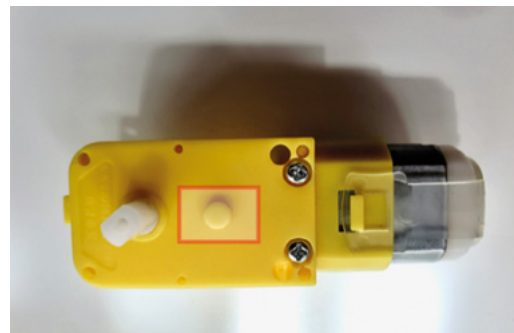
▲ Next to the axle, a motor has a knob (highlighted) to help align it. Include these in sketches as these will need holes too
