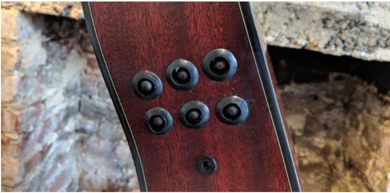
▲ The Braille reader on the other side of the guitar enables blind users to read instructions on how to play a chord
