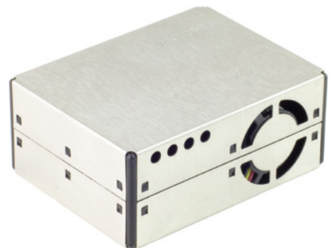
▲ Available separately, the PMS5003 sensor measures the number of tiny particles – up to 1, 2.5, and 10 microns – in the air
